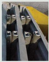
During head-on impacts at speeds up to 110 km/h, the QuadGuard CEN System telescopes rearward, crushing the cartridges and effectively dissipating the energy of both light cars (900kg) and large sedans (1500kg). During angle impacts at angles up to 15 degrees, the vehicles are safely redirected back into the original travel path.
